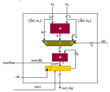
Figure 1: A digital design to be coded in RTL Verilog
